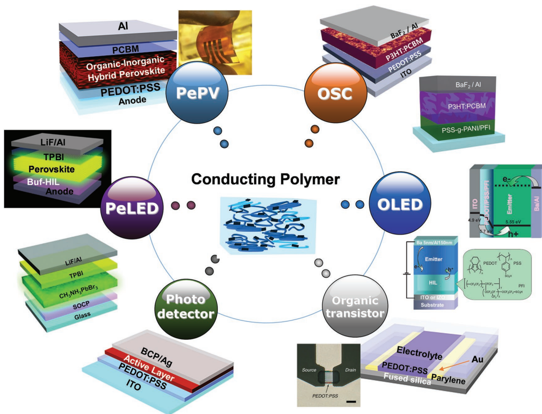
Figure 1. Applications of conducting polymers to organic and organic–inorganic hybrid perovskite electronics such as OSCs, upper image: Reproduced with permission. [10] Copyright 2014, WILEY-VCH. lower image: Reproduced with permission. [9] Copyright 2011, WILEY-VCH, OLEDs, Reproduced with permission. [4] Copyright 2007, WILEY-VCH, organic transistors, Reproduced with permission. [22] Copyright 2013, Nature Publishing Group, photo detector, PeLEDs, upper image: Reproduced with permission. [30] Copyright 2014, WILEY-VCH, lower image: Reproduced with permission. [31] Copyright 2015, American Association for the Advancement of Science, PePVs, right image: Reproduced with permission. [37] Copyright 2014, WILEY-VCH.
