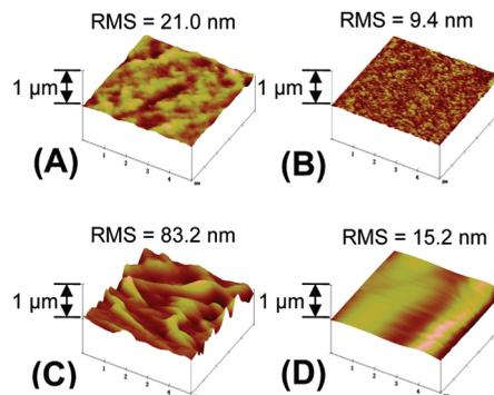
FIGURE 5. AFM topography images of the thin P3HT coatings with  $\text{FeCl}_3 \cdot 6\text{H}_2\text{O}$  on the glass substrate in cases of 5% EtOH/MeOH (A, before washing; B, after washing), 20% of the same solution with washing (C), and a 5% solution including isopropyl alcohol (D).
