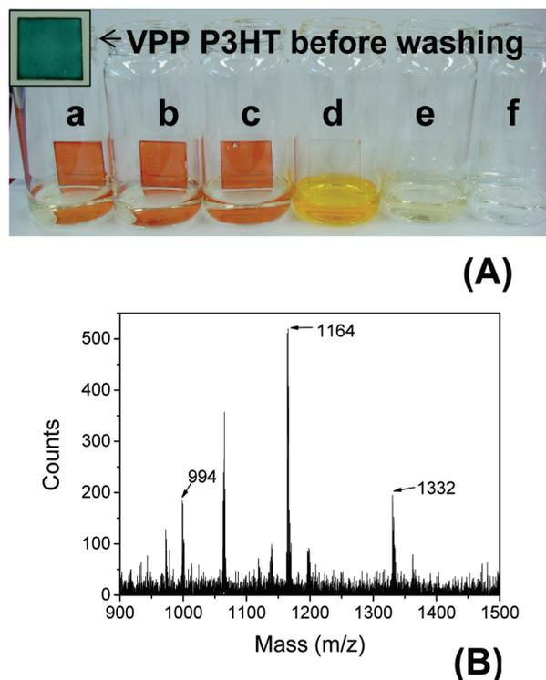
**FIGURE 3.** (A) Solubility test of a vapor-phase-polymerized P3HT coating on glass after being washed with MeOH for 3 h (a), 1 h (b), and 5 min (c) and washed with THF for 1 min (d), also exhibiting a  $\text{Fe}^{\text{III}}\cdot\text{Cl}\cdot 6\text{H}_2\text{O}$  coating (e) and monomer coating (f) on glass after being washed with MeOH for 1 min. (B) MALDI-MS spectrum of vapor-phase-polymerized P3HT at 55 °C for 1 h.
