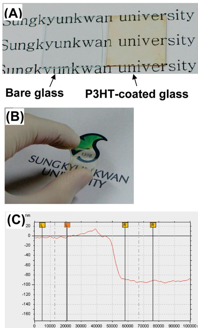
**FIGURE 2.** Images and an  $\alpha$ -step image of P3HT polymerized at 50 °C for 1 h: (A) comparison between vapor-phase-polymerized P3HT on glass and bare glass; (B) vapor-phase-polymerized P3HT coating with 90% optical transmittance on a flexible PET film; (C)  $\alpha$ -step image showing the thickness and morphology. Low levels were scraped off by a pincette.
