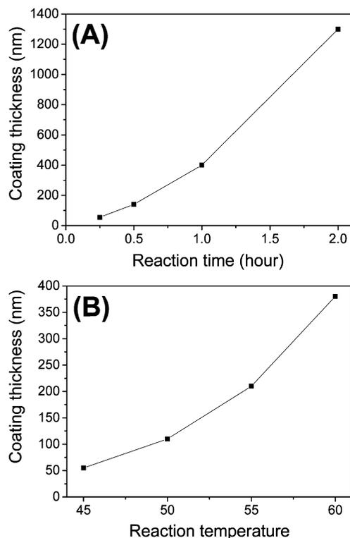
FIGURE 4. Vapor-phase-polymerized P3HT coating thickness as a function of the reaction time at 50 °C (A) and the reaction temperature for a 1 h reaction (B).
