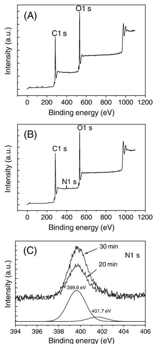
Fig. 1. XPS spectra of the untreated PET films (A), EDA-treated PET films (B), and the high-resolution XPS analysis of N1s peaks of EDA-treated PET films for different treatment times (C). The deconvoluted peaks of the EDA-treated PET for 20 min in (C) show amine and amide N–C bonds at 399.6 and 401.7 eV, respectively. All EDA treatments were performed at 40 °C.
