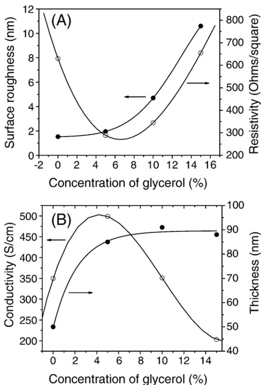
Fig. 8. Surface roughness and the surface resistivity of PEDOT-coated PET films (A), and the conductivity and thickness of PEDOT coating on glass substrates (B) as a function of glycerol concentrations at a fixed molar ratio of pyridine/Fe(OTs)<sub>3</sub> at 0.5.
