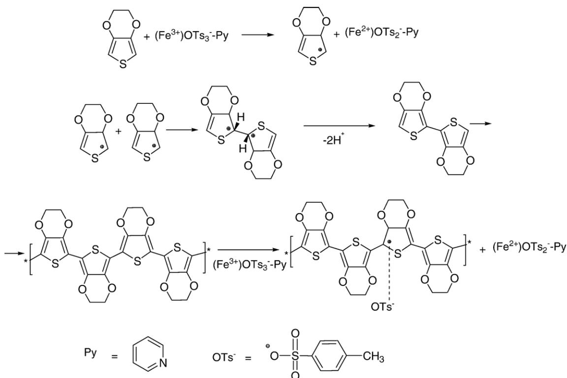
Scheme 2. Oxidative polymerization of EDOT in the presence of Py.
