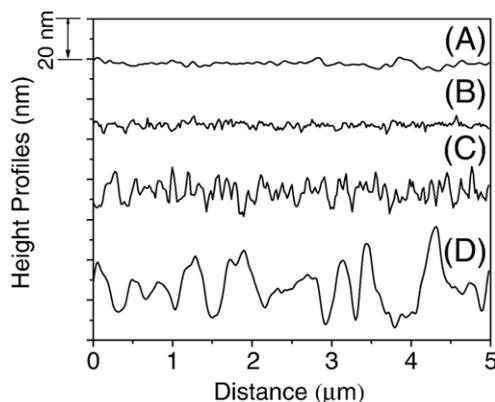
Fig. 10. AFM height profiles of PEDOT films at a fixed molar ratio of pyridine/Fe(OTs)<sub>3</sub> at 0.5 for various glycerol concentrations: (A) 0, (B) 5, (C) 10, (D) 15 wt.%.
