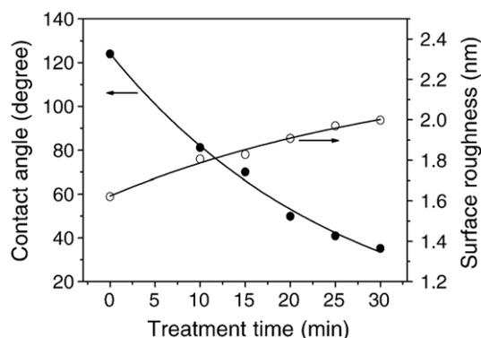
Fig. 2. Water contact angle and surface roughness of EDA-treated PET substrate films measured as a function of the EDA treatment time.
