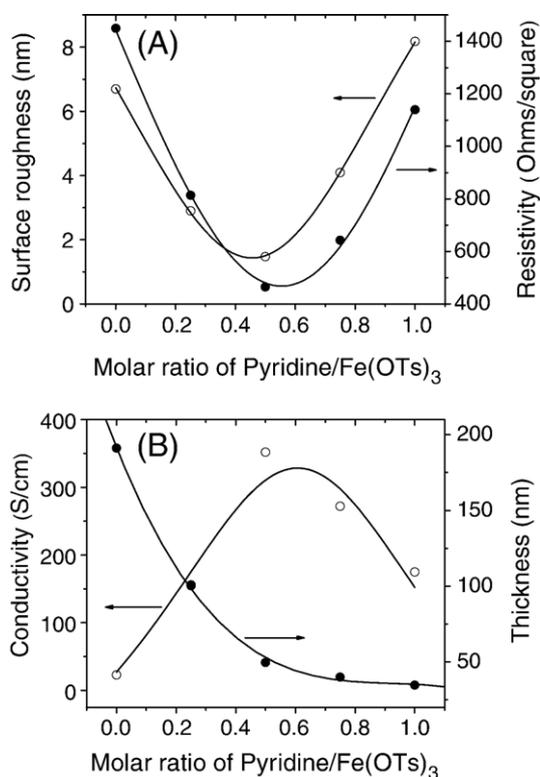
Fig. 4. Surface roughness and the surface resistivity of the PEDOT-coated PET films (A) to be compared with the conductivity and thickness of a PEDOT coating on glass substrates (B) at various molar ratios of pyridine/Fe(OTs)<sub>3</sub>.
