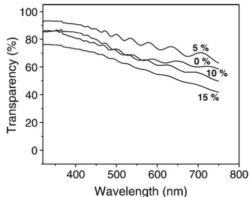
Fig. 9. Transparency of PEDOT films for various glycerol concentrations at a fixed molar ratio of pyridine/Fe(OTs)<sub>3</sub> at 0.5.
