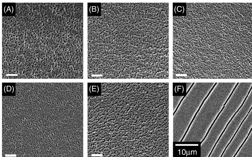
Fig. 3. FE-SEM images of PET film surfaces treated with EDA for (A) 0, (B) 15, (C) 20, (D) 25, (E) 30 and (F) 40 min at 40 °C in the gas phase. The scale bar represents 200 nm for A through E.
