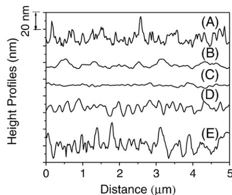
Fig. 5. AFM height profiles of PEDOT films at different Py/Fe(OTs)<sub>3</sub> ratios: (A) 0, (B) 0.25, (C) 0.5, (D) 0.75, (E) 1.0.
