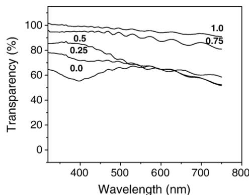
Fig. 6. Transparency of PEDOT films as a function of the pyridine/Fe(OTs)<sub>3</sub> molar ratio.
